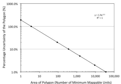
Figure 5 presents that for any given scale the level of uncertainty as function of the polygon size (in MMU). For instance if the objective is to obtain an uncertainty level lower than 5%, then the size of a square polygon should be around 360 MMU or more. For areas larger than 10,000 times the MMU uncertainty will be below 1%. In the context of CBM this means that if relatively small polygons are mapped with high errors, the associated uncertainty of the geographical information will be high.
